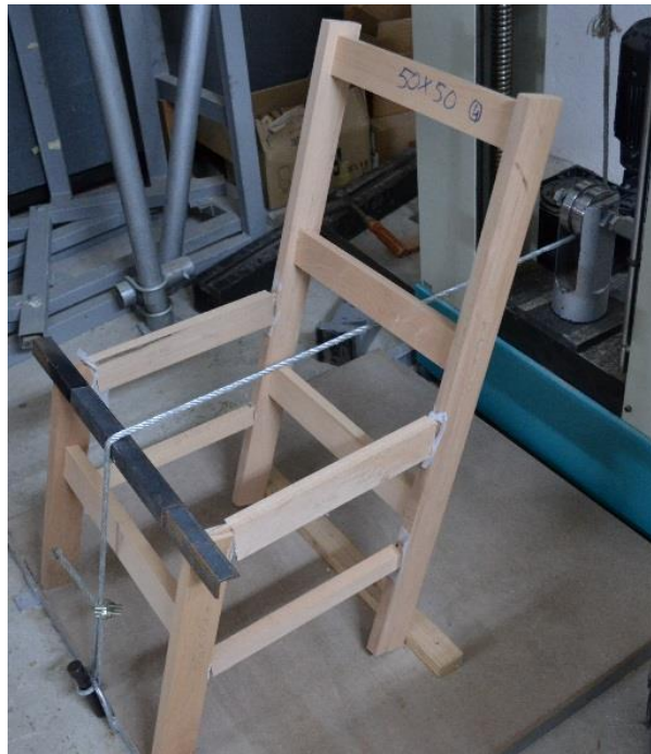
Fig. 5. The general failure modes of the chair frames after static front to back loading test
