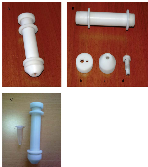
Fig. 1 A) Biocentri-voltammetric cell, B) Parts of the biocentri-voltammetric cell: body (a), cover for reference and counter electrode (b), protective cover for working electrode (c) and carbon paste working electrode (d), C) Eppendorf tube with the voltammetric cell, scale (1 : 2).
