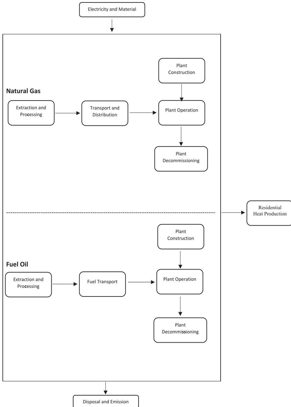
**Figure 1.** System boundary of LCA study.
