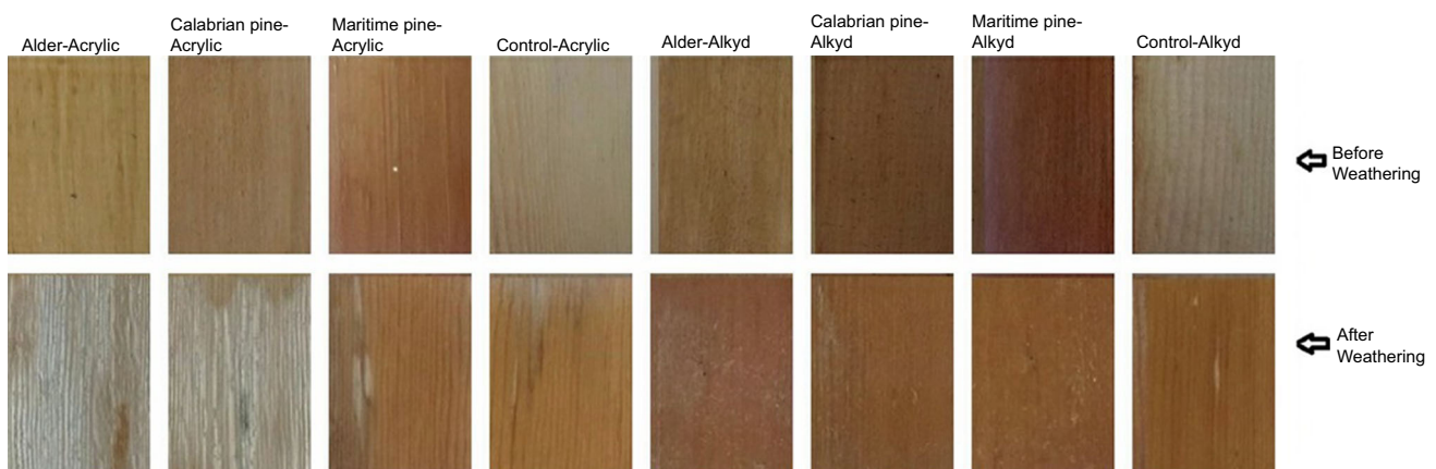
Fig. 8: Appearance of samples applied with alkyd- and acrylic-based coating systems
