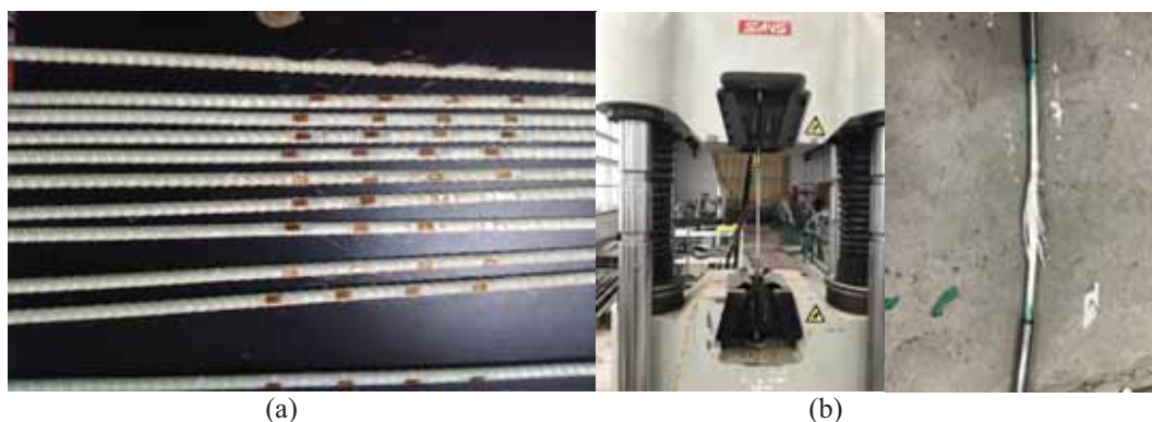
FIGURE 4 GFRP rods and tensile test. (a) GFRP rods; (b) Tensile test
