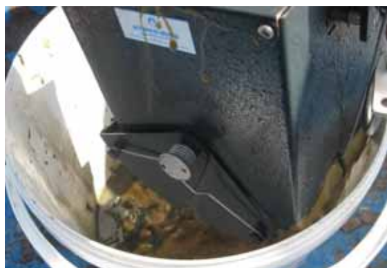
FIGURE 3A Sediment taken with the Ekman-Birge sampler
