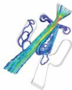
FIGURE 3 Particle trajectory in the jet element.
