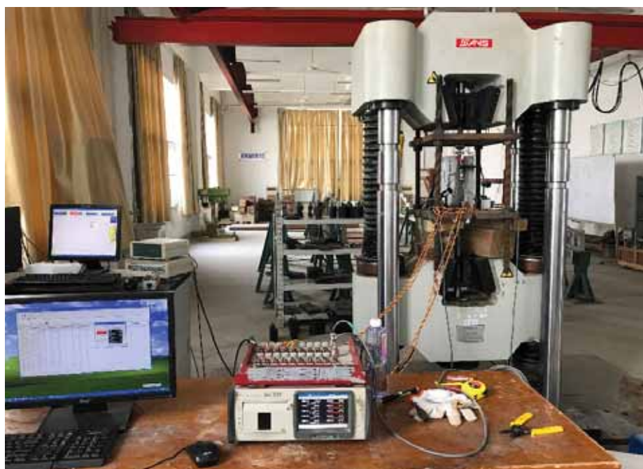
FIGURE 7 Pull-out test setup
